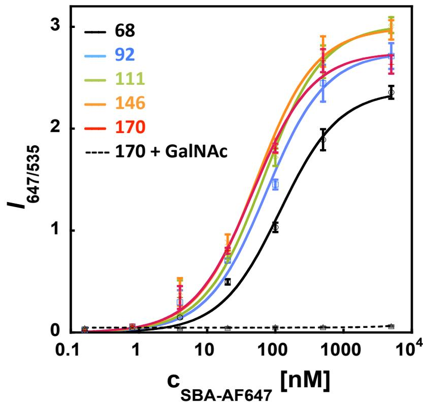
$$I_{647/535,\text{obs}} = \frac{I_{647/535,\text{max}}}{\frac{K_d}{[L]} + 1}$$
